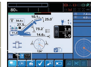
Preset menu display (during crane operation)
