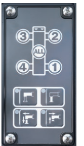
Outrigger Control Panel
